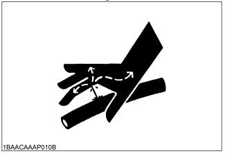
16. Fluid escaping from pinholes may be invisible. Do not use hands to search for suspected leaks; use a piece of cardboard or wood. Use of safety goggles or other eye protection is also highly recommended. If injured by escaping fluid, see a medical doctor at once. This fluid will produce gangrene or severe allergic reaction.
