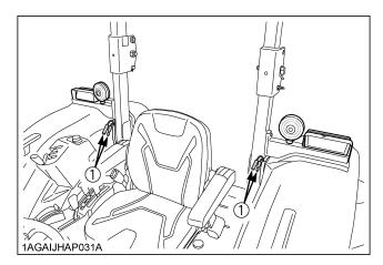
(1) Accessory electrical outlet for rear work light (35W)
