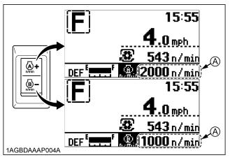
(A) Light up.... Engine revolution is operating in the rpm memory setting value.
