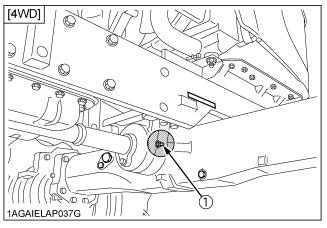
(1) Grease fitting (Front axle support)
