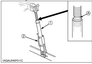
(1) Lifting rod (2) Adjusting handle
