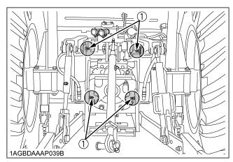
(1) Grease fitting (Hydraulic lift cylinders pin)
