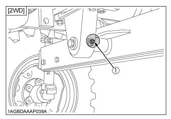
(1) Grease fitting (Front axle support)
