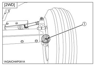
(1) Grease fitting (Knuckle shaft) [RH, LH]
