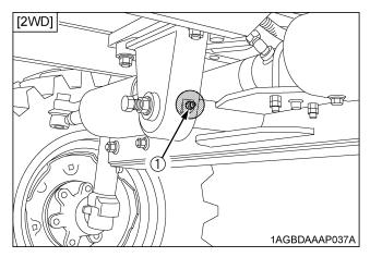
(1) Grease fitting (Front axle support)
