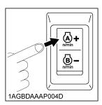
Again press and hold down the switch (A) side (2.5 seconds) until the buzzer sounds, then release the switch.
