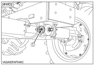
(1) Grease fitting (Front axle support)
