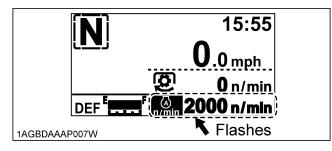
Press the switch to the (A) or (B) side and set the speed.
