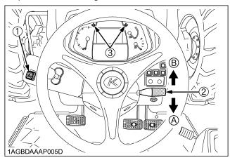
(1)Hazard light switch (2)Turn signal light switch (3)Hazard / Turn signal indicator
