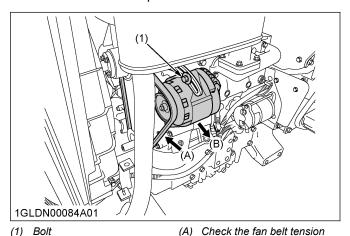
4. Replace the fan belt if it is damaged.
