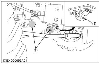
(1) Grease fitting (front axle sup- (2) Breather plug
