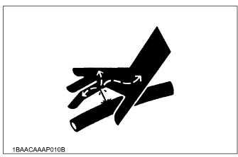
Hydraulic fluid escaping from pinholes may be invisible. Do not use hands to search for suspected leaks. Use a piece of cardboard or wood to search for suspected leaks. You should use safety goggles or other eye protection. If injured by escaping fluid, see a medical doctor at once. Hydraulic fluid will produce gangrene or severe allergic reaction.
