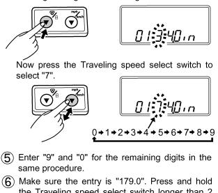
b) Make sure the entry is 179.0. Press and hold the Traveling speed select switch longer than 2 seconds. The setting is put in memory, and the LCD monitor goes back to the Hour meter mode.
