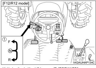
(1) Hydraulic-shuttle shift lever (2) Main gear shift lever
