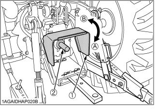
(1) PTO Shaft cover (2) PTO Shaft cap
