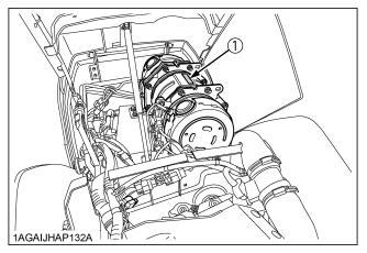
(1) Diesel Particulate Filter (DPF) serial number
