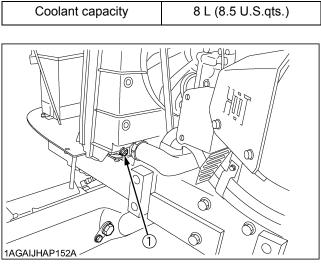
(1) Drain plug ((+) Plus screwdriver)
