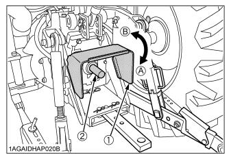
(1) PTO shaft cover(2) PTO shaft cap
