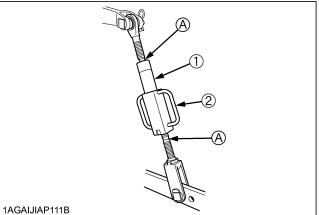
(1) Lifting rod (2) Adjusting handle
