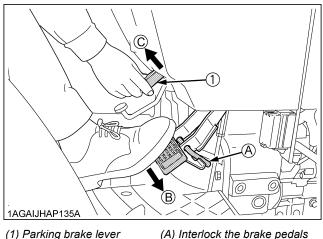
(1) Parking brake lever (A) Interlock the brake pe (B) "DEPRESS" (C) "PULL"
