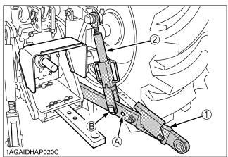
(1) Lower link (2) Lifting rod holes: (A), (B)
