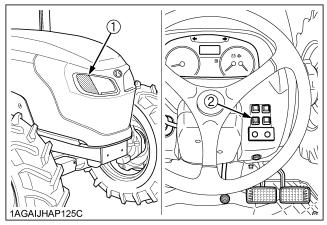
(1) Front work light(2) Front work light switch with indicator
