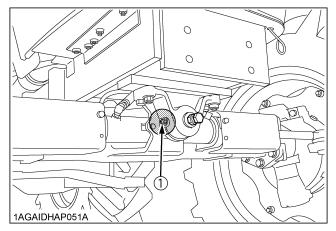
(1) Grease fitting (Front axle support)
