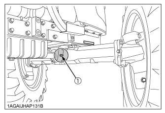
(1) Grease fitting (Front axle support)
