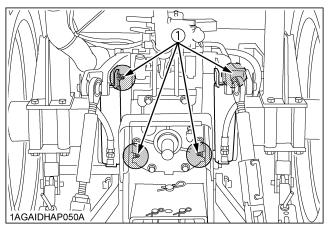
(1) Grease fitting (Hydraulic lift cylinders pin)
