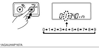
(4) Press the PTO/Hour meter select switch, and the next highest digit starts flashing.
