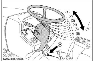
(1) Steering wheel tilt pedal (A) "PRESS DOWN"
