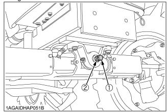
(1) Adjusting screw (2) Lock nut
