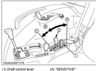
(1) Draft control lever (2) Position control lever (A) "SENSITIVE"(B) "INSENSITIVE"(C) "FLOAT"
