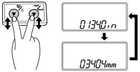
(3) Note that the highest-digit numeral is flashing. Press the Traveling speed select switch to select "1". (The numeral changes from 0 to 9 at each push of the switch.).
