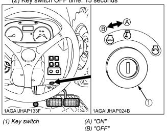
3. Set the hand throttle lever at the maximum speed position, turn the key switch to start the engine and then reset the throttle lever at the mid speed (around 1500 rpm) position.
