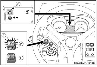
(1) 4WD switch with indicator (A) 4WD "ON" (2) 4WD indicator (B) 4WD "OFF"
